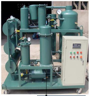
Decolorization system, with high absorbability, it can change the color and absorb the dissolved particles
